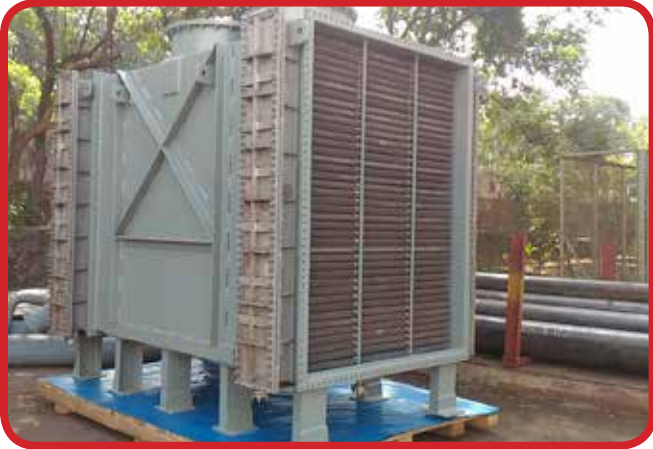
PUMP ROOM COOLER
