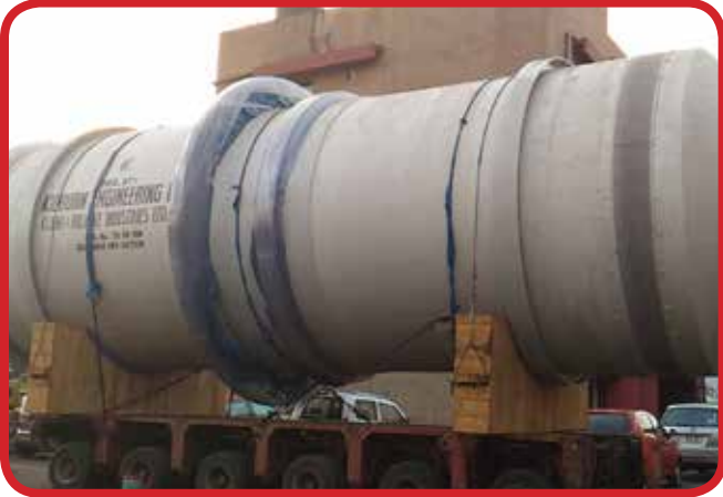
ROTARY DRYER SECTION-I
