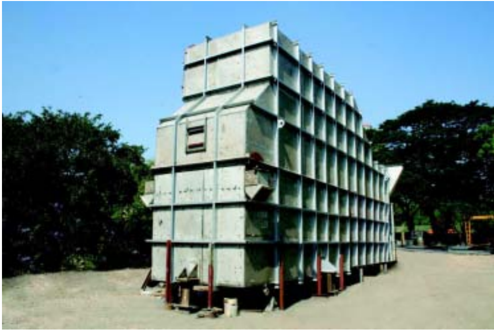
Fluid Bed Cooler for a Fertilizer Plant
